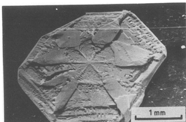
Figure 2 SEM photograph of BiSI single crystal.
